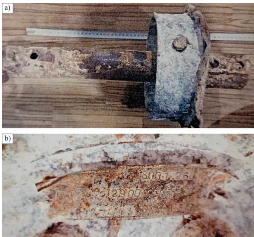
Fig. 22. Włostów, Opatów district. Suspension component from the wheels of a German RSO artillery tractor – Steyr Raupenschlepper Ost: a) before exploration; b) after exploration; c) reference photo. Photo from the Historical and Exploratory Association “Pamięć” 2024
